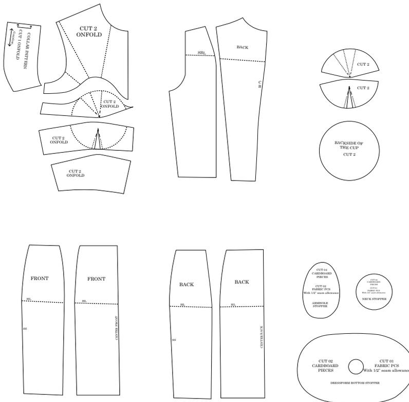
**Figure 1:** Pattern components of half scale dress form
